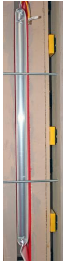
Model 2 Joint width 6 cm, vertical shear
