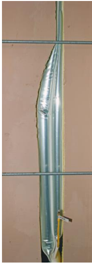
Model 1 Joint unevenness 2 to 8 cm over a length of ~ 40 cm
