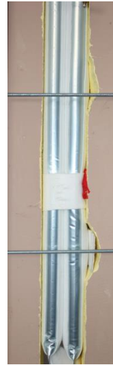
Model 3 Joint width 12 cm, uneven places, concrete chipped with/out residue
