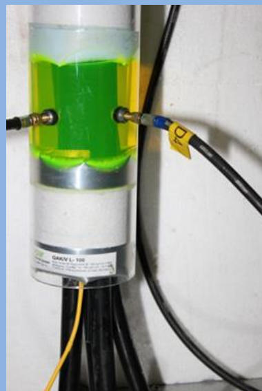
5 m water column on the test specimen
